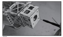
36 Install the motor mount to the fuselage.
