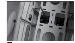
33 Secure the landing gears to the fuse by screws provided.
