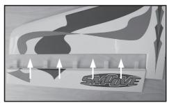
Use CA with accelerator to glue in the 1 aileron hinges (be careful not to bind the hinges up with excessive glue).
