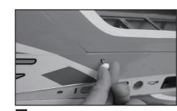
44 Secure the canopy by thumb screws.
