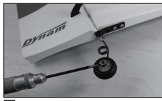
19 Tighten collet to secure the wheel in position.
