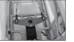
Attach the ball link to the rudder servo 27 horns making sure the wires are tight and not slack
