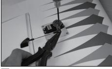
6 Install the servo push rod/links.
