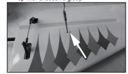
22 Use a 1.6mm drill to drill the marked position on the elevator.
