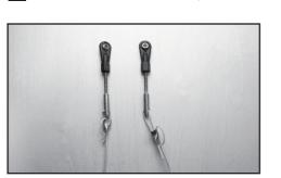
26 Install rudder push/pull ball link to the wire.
