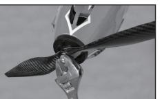
41 Install the propeller.
