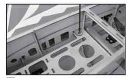
43 Install the left and right wing in place and secure to fuselage by screws.
