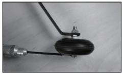
**30** Tighten the collet to secure the wheel in position.
