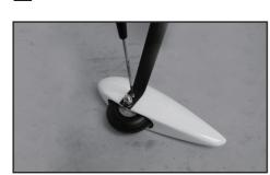
32 Secure the wheel pant with screws provided.
