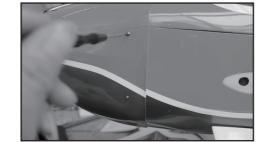
39 Align and secure the cowl to the fuse with screws.
