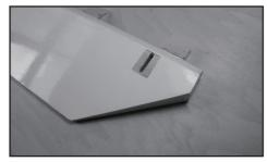
8 Cut out the slot for the servo horn position.
