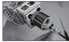
37 Install the motor to the motor mount.
