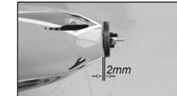
40 Install the backing for the spinner, making sure there is a 2mm clearance gap.
