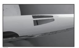
20 Cut out the bottom air cooling outlet
