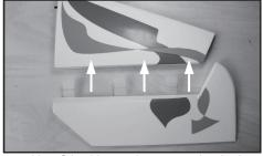
Use CA with accelerator to glue in the 7 elevator hinges (be careful not to bind the hinges up with excessive glue).
