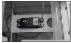
25 Install the Rudder servo in position.
