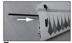
21 Install the Rod into the elevator
